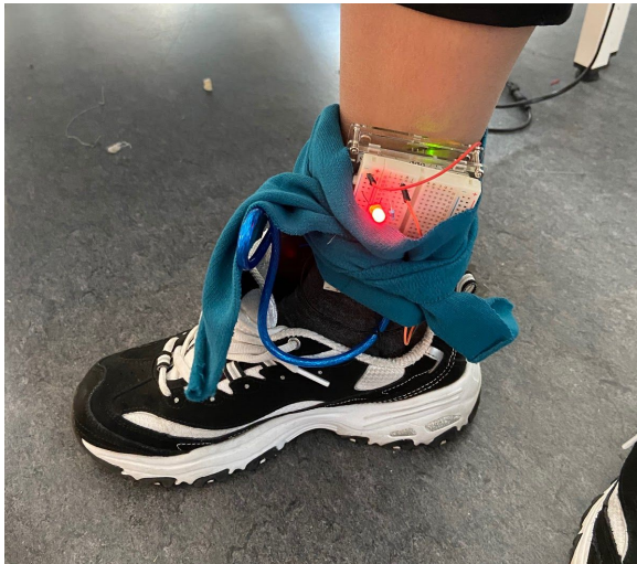
Early prototype, testing the sensitivity of a pressure sensor using a led light.
