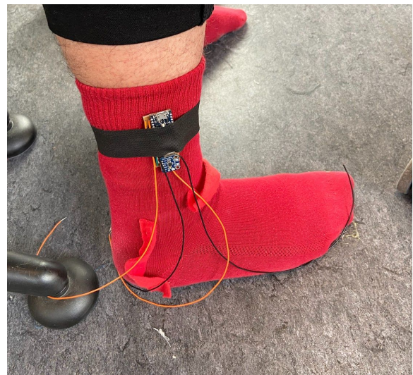
Sock prototype without the pressure sensor and vibration motor.
